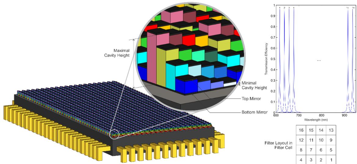
*Figure 10: A schematic representation of an integrated implementation of the Fabry-Pérot optical filter on top of standard CMOS imager in a pixel-level mosaic layout (dimensions not to scale, left) and alignment of filters to pixels (right) [17].*
