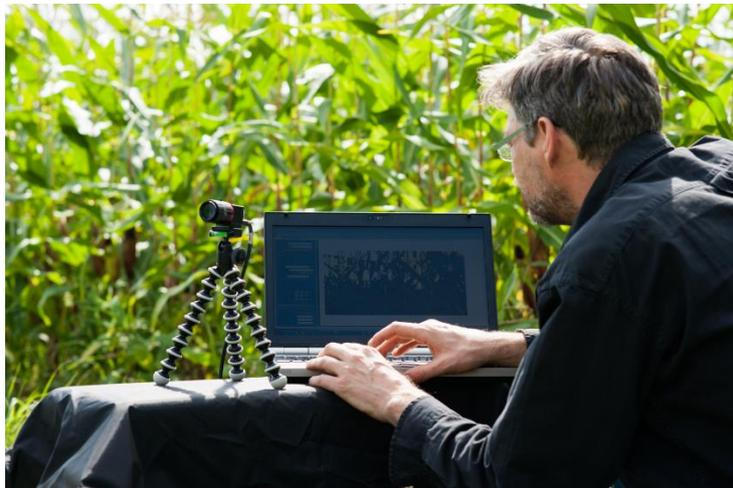
*Figure 14: The tiny size of the xiQ camera enables flexible outdoor spectral data acquisition.*
