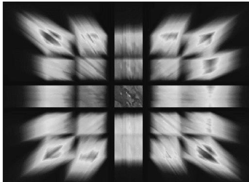
Figure 2: CTIS tomographic dispersion pattern, showing a complex landscape in panchromatic 0th order in the center, while angular chromatic dispersion creates the surrounding higher orders [3].
