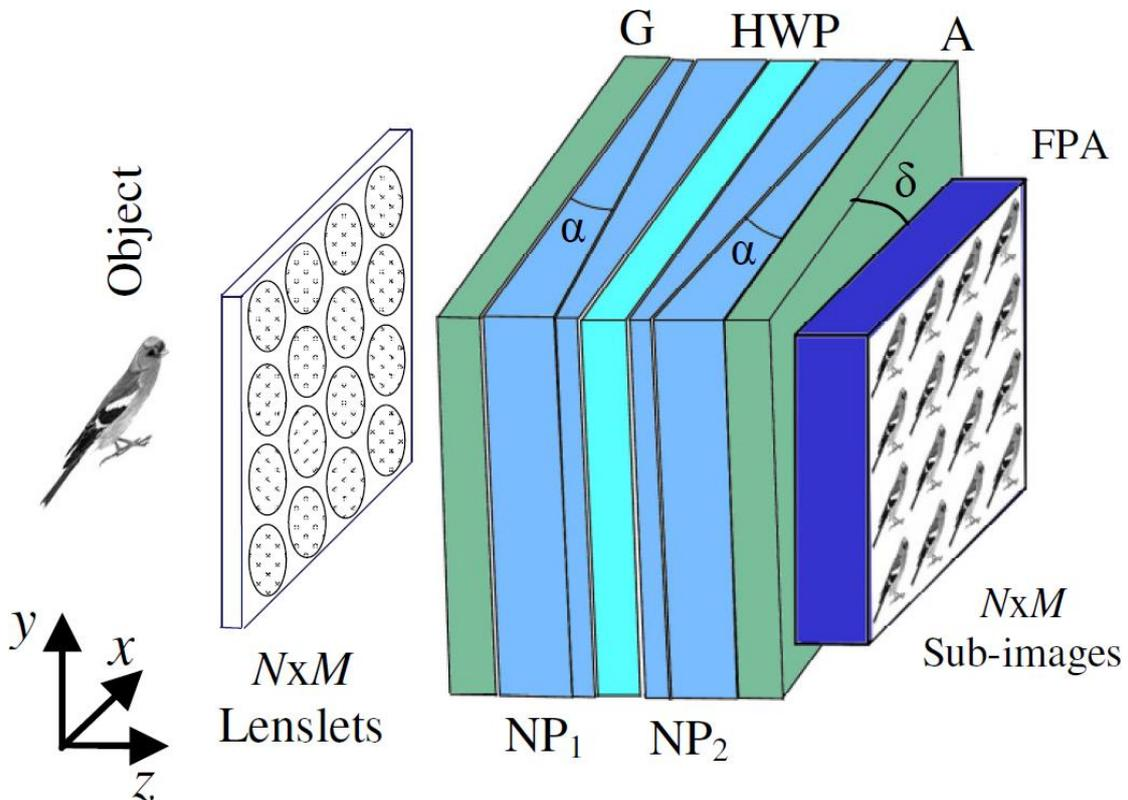
Figure 7: Snapshot Hyperspectral Imaging Fourier Transform Spectrometer or SHIFT, including a lenslet array, G(enerating) and A(nalyzing) Polarizers, two birefringent Nomarski Prisms (NP) and a Half-Wave Plate (HWP) in front of a focal plane array (FPA) [11]
