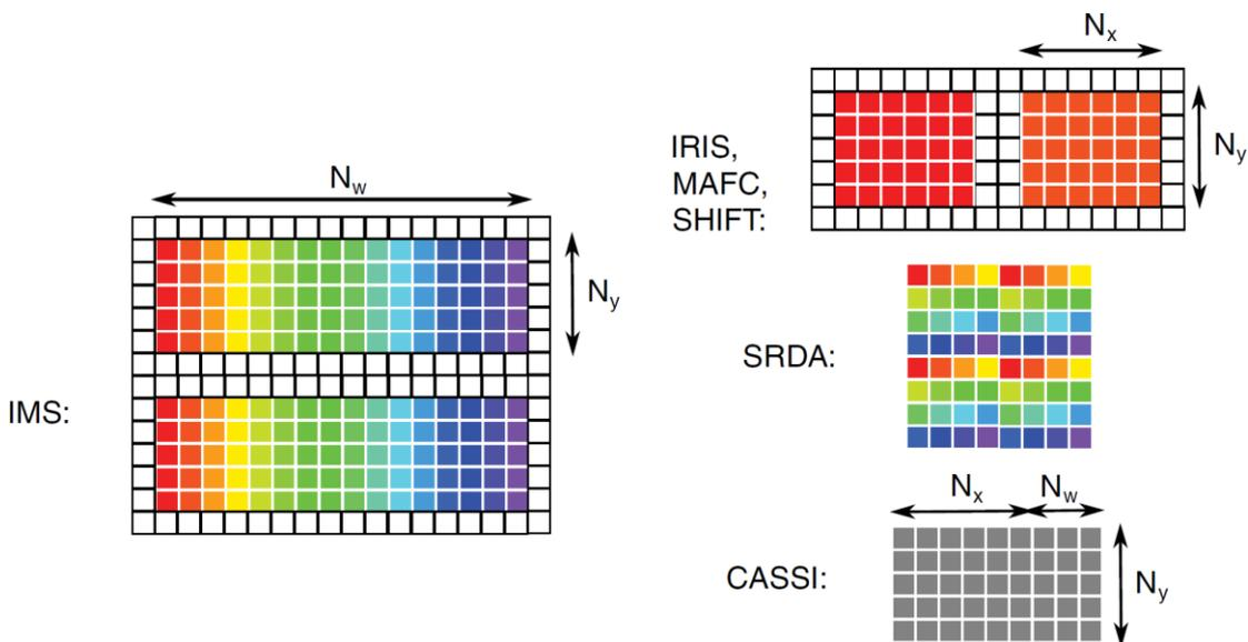
Figure 11: Diagrams showing how the detector utilization formulas are calculated for each architecture, given the basic layout of how the datacube projected onto the two-dimensional detector array. Each square shown here represents a single pixel on the detector array [18].
