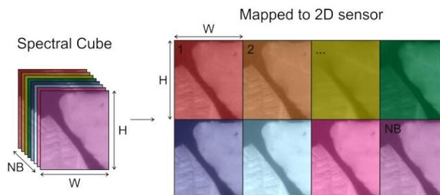
Figure 12: Spectral cube with NB bands and spatial resolution of  $W \times H$  mapped to NB tiles on 2D sensor.
