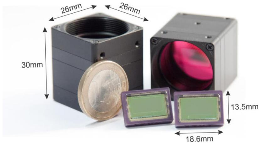
*Figure 13: Two packaged mosaic spectral snapshot sensors, alongside two tiny spectral cameras and a euro coin for scale.*
