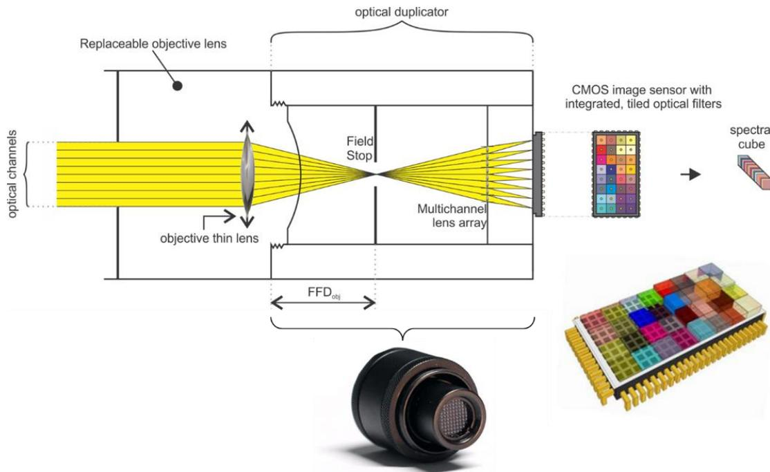
Figure 8: imec snapshot tiled, where scene simultaneously and fully duplicated on each filter tile using optical duplication [16].
