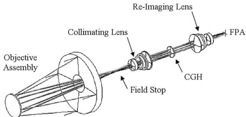
Figure 3: Generalized optical layout of CTIS [3]
