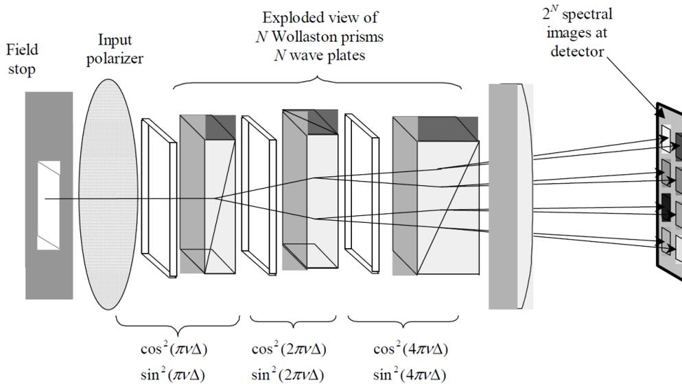
Figure 6: Depiction of principle of operation of Image replication imaging spectrometer (IRIS, [8]).
