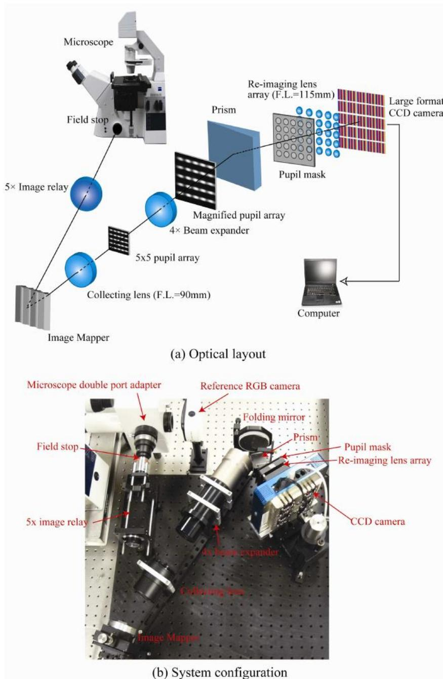
Figure 5: IMS Optical layout and system prototype configuration [6].
