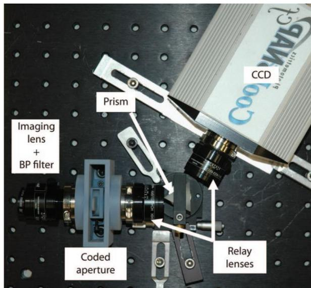
Figure 4: Experimental prototype of the SD (Single Disperser) CASSI [5].
